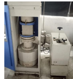
figure 3.5 Concrete cubes testing
