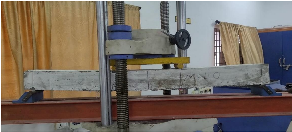
Figure 3.9 Flexural Strength Test on Beam
